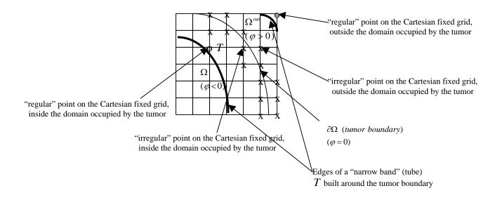
Fig. 1 Schematic of the tumor boundary representation in the Cartesian grid, "narrow band" level set approach.
