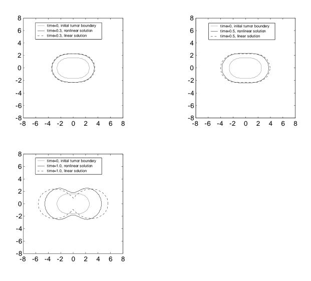
**Fig. 4.** Comparison between the nonlinear solution obtained via the narrow band level set approach and the solution obtained using the linear analysis developed in [1] for the low vascularization regime (G=20, A=0.5). Initial tumor boundary given by Eq. (5.1). Mesh size h = 0.18 and time step  $\Delta t = 0.001$ .
