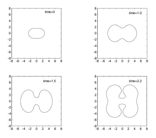
**Fig. 5.** Nonlinear tumor evolution in time via the narrow band level set approach (WENO) for the low vascularization regime (G=20, A=0.5). Initial tumor boundary given by Eq. (5.1). Mesh size h = 0.09 and time step  $\Delta t = 0.00025$ .
