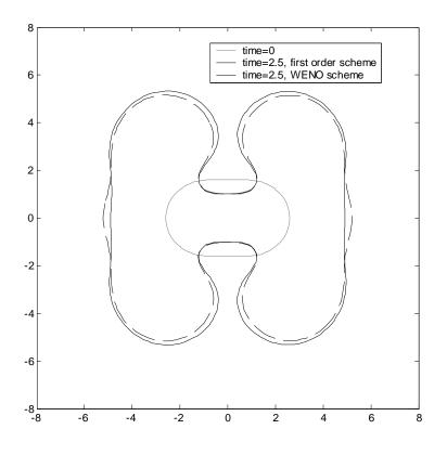
**Fig. 3.** Comparison of nonlinear tumor evolution in time obtained employing a first-order level set scheme vs. a WENO scheme; the solution obtained via the first-order scheme exhibits numerical dissipation. Initial tumor boundary given by Eq. (5.1), low vascularization regime (G=20, A=0.5). Mesh size h = 0.18 and time step  $\Delta t = 0.001$ .
