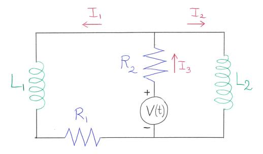
in which  $R_1 = 8$  ohms,  $R_2 = 4$  ohms,  $L_1 = 2$  henries,  $L_2 = 1$  henry.
